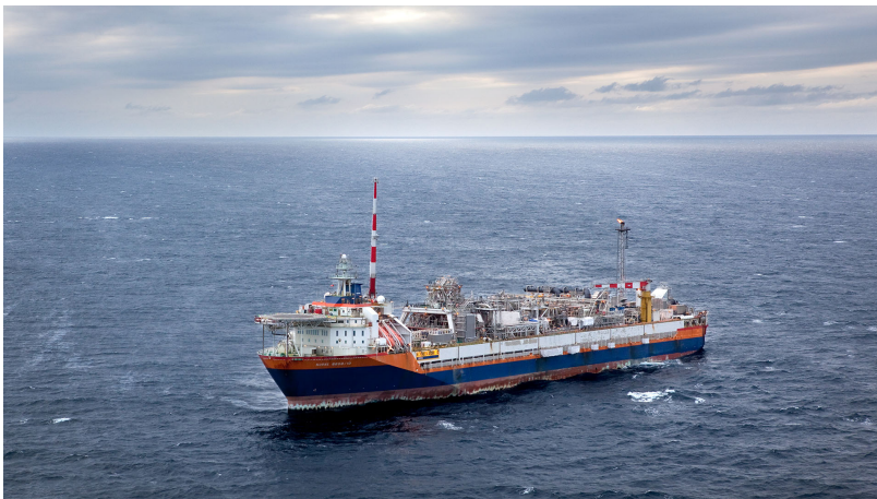
Figure 14.1: A picture of the Norne FPSO; Norneskipet. The ship was built in Singapore, and has a storage capacity of 115 thousand ton. The gas flare can be seen at the stern of the ship. (Foto: Equinor.)
